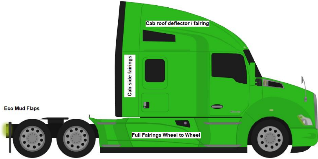
Image 4: Cab roof deflector/fairing, Cab side fairings, Full fairings wheel to wheel, Eco Mud Flaps
