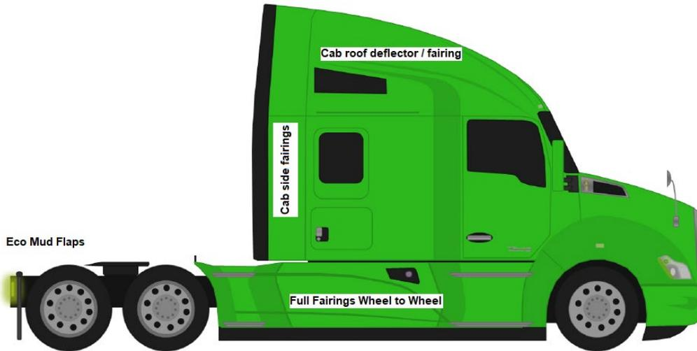
Image 5: Cab Roof Fairing (non-adjustable)
